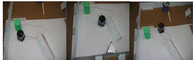
Fig. 5. Autonomous obstacle avoidance. The robot approaches an obstacle, stops, reverses, and turns away
