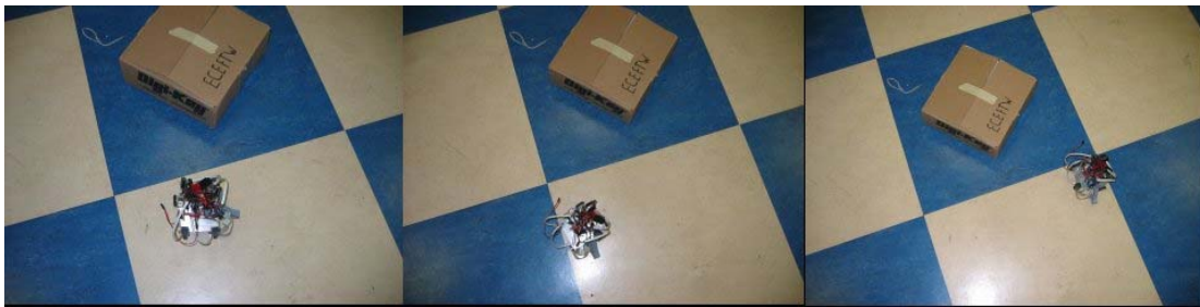
Figure 4. Autonomous Obstacle avoidance using a SMARbot
