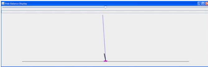
Fig. 3. Double pole balance simulator GUI display. The pink block represents the cart. The navy and blue poles indicate the deflection from vertical of the short and long pole, respectively. The line beneath the cart is the track. Letting a pole fall more than 36^\circ from vertical or running off of the track constitutes failure. To prove itself to be a valid solution, an ANN must pass 10 trials, each lasting 100,000 simulation steps.
