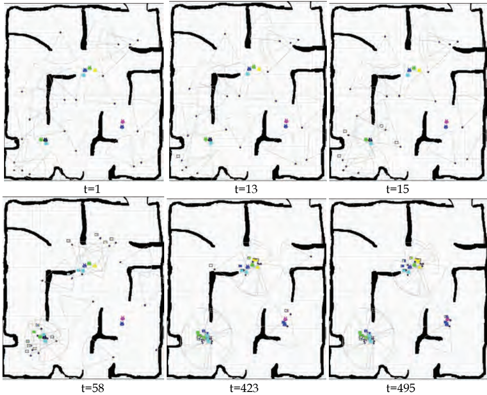
Figure 3. 20 robots search for randomly distributed targets in an indoor office environment on a player/stage simulator at t = 1, 13, 15, 58, 423, and 495 time steps
