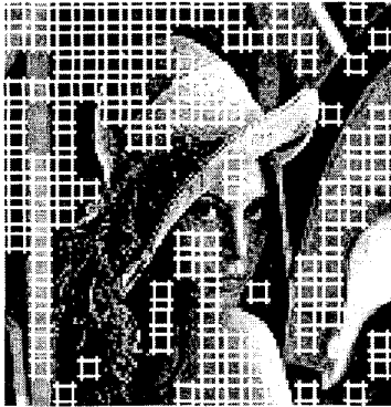
Figure 4: Watermarked blocks for the Lena image are shown as white squares. These blocks and the watermark energy were chosen based on the proposed iterative waterfilling algorithm.
